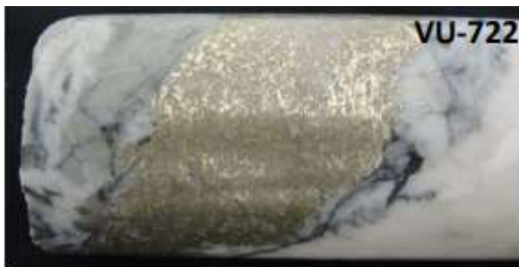
Figure 1: Drill core from Pretium's Valley of the Kings grading 42,100 gpt Au (1,353 oz).
